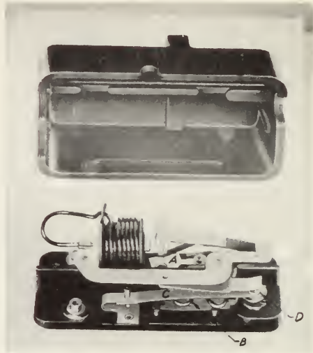
6-40. An amperage-magnetic relay. This control keeps the starting winding points open by means of a cantilever spring. Only when current first flows through the magnetic coil is the magnetism powerful enough to lower the spring and close the starting circuit at "A." If the unit consumes too much current, the resistance wire coil "B" will heat and bend the bimetal strip "C" and open the circuit at "D."
